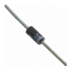
1N4750APE3/TR12 Microsemi Corporation DIODE ZENER 27V 1W DO204AL
