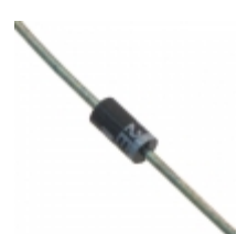
1N4750AP/TR12 Microsemi Corporation DIODE ZENER 27V 1W DO204AL
