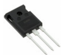
IXFH15N80Q IXYS MOSFET N-CH 800V 15A TO-247AD
