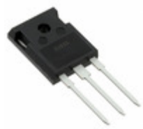
IXFH15N60 IXYS MOSFET N-CH 600V 15A TO-247AD
