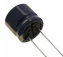
EEU-FC1C332SB Panasonic Electronic Components CAP ALUM 3300UF 20% 16V RADIAL
