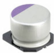
16SVP100M Panasonic Electronic Components CAP ALUM POLY 100UF 20% 16V SMD
