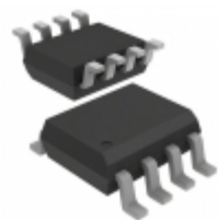
ADM13307-25ARZ-RL7 Analog Devices Inc. IC SUPERVISOR MCU 3CH 8SOIC
