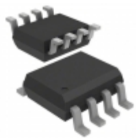
ADM13305-4ARZ Analog Devices Inc. IC SUPERVISR DUAL 3.3/ADJ 8SOIC
