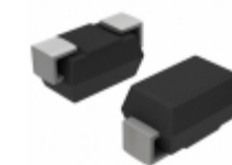
SMAJ200A-H Bourns Inc. TVS DIODE 200VWM 324VC DO214AC
