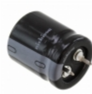
LLS2Z391MELZ Nichicon CAP ALUM 390UF 20% 180V SNAP
