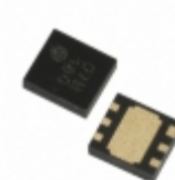
XC6122A635ER-G Torex Semiconductor Ltd IC WATCHDOG TIMER 6-USP
