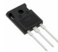
IXFH13N100 IXYS MOSFET N-CH 1000V 12.5A TO-247
