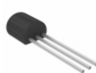
BC559_J35Z AMI Semiconductor / ON Semiconductor TRANS PNP 30V 0.1A TO-92
