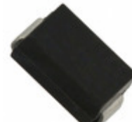
P4SMA18A_D84Z Fairchild/ON Semiconductor TVS DIODE 15.3VWM 25.2VC SMA
