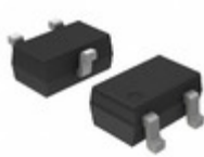
BC857BWT1 ON Semiconductor TRANS PNP 45V 0.1A SOT-323
