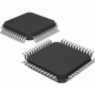
LC4032B-10TN48I Lattice Semiconductor Corporation IC CPLD 32MC 10NS 48TQFP
