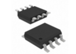
AO4433 Alpha & Omega Semiconductor Inc. MOSFET P-CH 30V 11A 8SOIC
