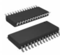
PIC16C642-04I/SO Microchip Technology IC MCU 8BIT 7KB OTP 28SOIC
