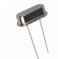
ATS400B-E CTS-Frequency Controls CRYSTAL 40.0000MHZ 18PF T/H
