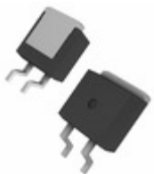
IXFA7N80P IXYS MOSFET N-CH 800V 7A TO-263
