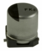
EEE-FK1K3R3R Panasonic Electronic Components CAP ALUM 3.3UF 20% 80V SMD
