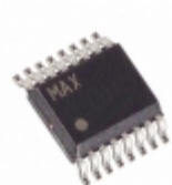
MAX1701EEE+ Maxim Integrated IC REG BOOST ADJ 1.1A 16QSOP
