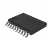
CS4352-DZZR Cirrus Logic Inc. IC DAC STER 102DB 192KHZ 20TSSOP
