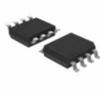
BR24S128FJ-WE2 Rohm Semiconductor IC EEPROM 128KBIT 400KHZ 8SOP-J
