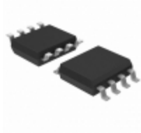
BR24S16F-WE2 Rohm Semiconductor IC EEPROM 16KBIT 400KHZ 8SOP
