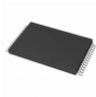
AT28BV16-25TC Microchip Technology IC EEPROM 16KBIT 250NS 28TSOP
