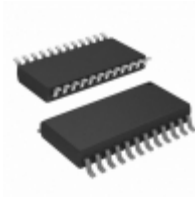
AT28BV16-25SI Microchip Technology IC EEPROM 16KBIT 250NS 24SOIC
