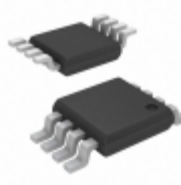
PAM2401SCADJ Diodes Incorporated IC REG BOOST ADJ 3A SYNC 8MSOP
