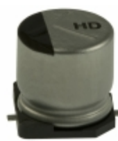
EEE-HD1V330AP Panasonic Electronic Components CAP ALUM 33UF 20% 35V SMD
