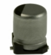
ECE-V1AA330NP Panasonic Electronic Components CAP ALUM 33UF 20% 10V SMD
