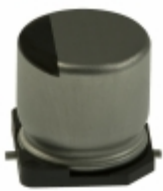
EEE-HA1C221UP Panasonic Electronic Components CAP ALUM 220UF 20% 16V SMD
