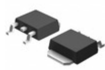
RD3T100CNTL1 LAPIS Semiconductor NCH 200V 10A POWER MOSFET
