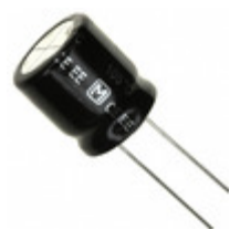
EEU-EE2D101S Panasonic Electronic Components CAP ALUM 100UF 20% 200V RADIAL
