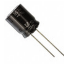
EEU-EE2D151 Panasonic Electronic Components CAP ALUM 150UF 20% 200V RADIAL
