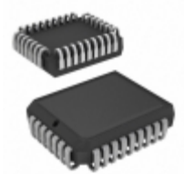
AT28HC256F-70JI Microchip Technology IC EEPROM 256KBIT 70NS 32PLCC
