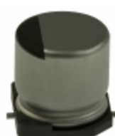
EEE-HAA330WAR Panasonic Electronic Components CAP ALUM 33UF 20% 10V SMD
