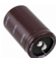
EKMH630VNN103MA50T United Chemi-Con CAP ALUM 10000UF 20% 63V SNAP
