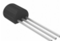
S-812C25AY-Z2-U SII Semiconductor Corporation IC REG LINEAR 2.5V 30MA TO92
