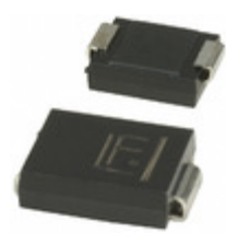
SMCJ54A Littelfuse Inc. TVS DIODE 54VWM 87.1VC SMC
