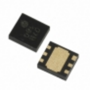
XC6123C322ER-G Torex Semiconductor Ltd IC WATCHDOG TIMER 6-USP
