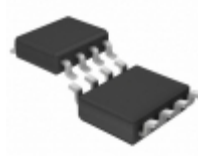
LT1461CIS8-5#PBF ADI (Analog Devices, Inc.) IC VREF SERIES 5V 8SOIC
