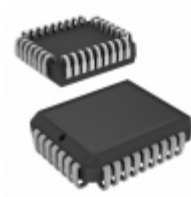
AT27C080-90JI Microchip Technology IC OTP 8MBIT 90NS 32PLCC
