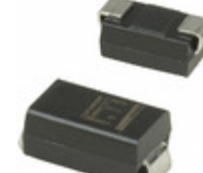
SMAJ54A Littelfuse Inc. TVS DIODE 54VWM 87.1VC SMA
