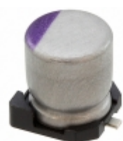
20SVPF56MX Panasonic Electronic Components CAP ALUM POLY 56UF 20% 20V SMD
