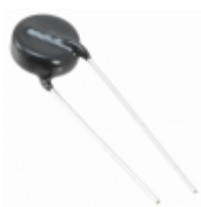
ERZ-E11A751CS Panasonic Electronic Components VARISTOR 750V 5KA DISC 14MM
