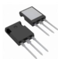
IXFR20N100P IXYS MOSFET N-CH 1000V 11A ISOPLUS247
