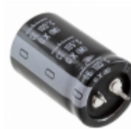
LGX2E681MELA40 Nichicon CAP ALUM 680UF 20% 250V SNAP
