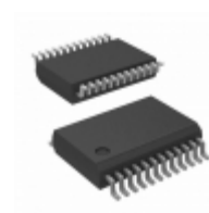
LC87FBG08AUJA-TLM-H ON Semiconductor IC MCU 8BIT 8KB FLASH 24SSOP
