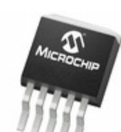
MCP1827T-1802E/ET Microchip Technology IC REG LDO 1.8V 1.5A DDPAK
