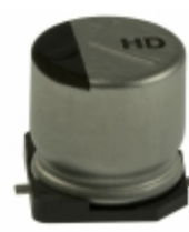
EEE-HD1J100P Panasonic Electronic Components CAP ALUM 10UF 20% 63V SMD
