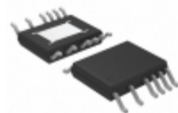
LTC3639HMSE#PBF ADI (Analog Devices, Inc.) IC REG BUCK ADJ 0.1A SYNC 16MSOP
