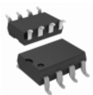
ACPL-827-36BE Broadcom Limited OPTOISOLATOR 5KV 2CH TRANS 8SMD
