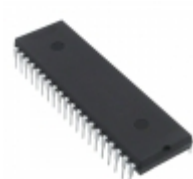
AT89LP51-20PU Microchip Technology IC MCU 8BIT 4KB FLASH 40DIP
