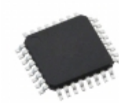
AT89LP428-20AU Microchip Technology IC MCU 8BIT 4KB FLASH 32TQFP
