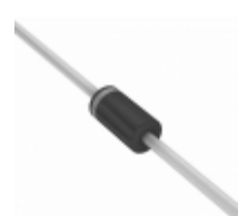
BZW04-70B A0G TSC (Taiwan Semiconductor) TVS DIODE 70.1V 113V DO204AL
