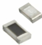
RR0816P-622-B-T5 Susumu RES SMD 6.2K OHM 0.1% 1/16W 0603
