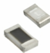
RR0816P-6490-D-79A Susumu RES SMD 649 OHM 0.5% 1/16W 0603
