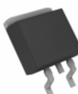
BA7807FP-E2 Rohm Semiconductor IC REG LDO 7V 1A TO252-3
